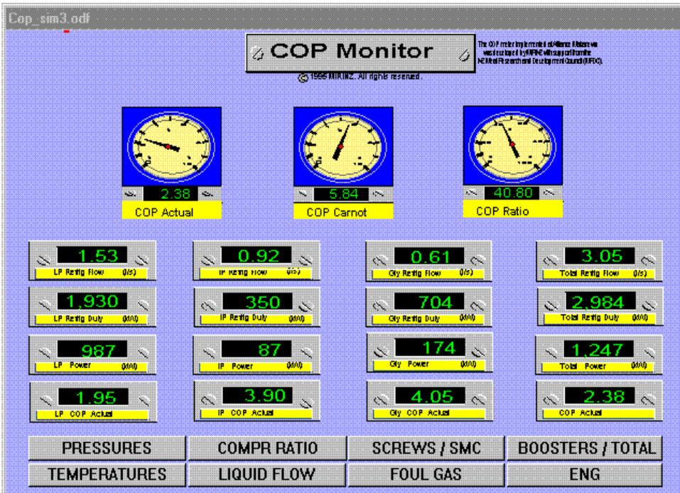
The COP monitor measures refrigerant flows, calculates refrigeration system efficiency, and shows data clearly and in a useful format
